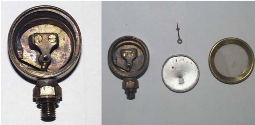
The beginning and end of the hollow spring are soldered. These points can be leaking air. Any adjustment or calibration, is not possible.
