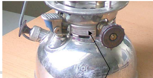
Pict. 38. Cooling ribs
